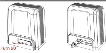
To make the motor into manual mode, insert the key and open the manual release bar till it rotates by  $90^{\circ}$ .
