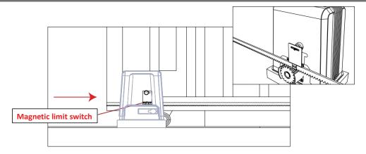
Test the spring/magnetic limit switch stops by moving the gate manually until you hear a click, making sure contact is made with the spring/magnetic limit switch on the motor.
