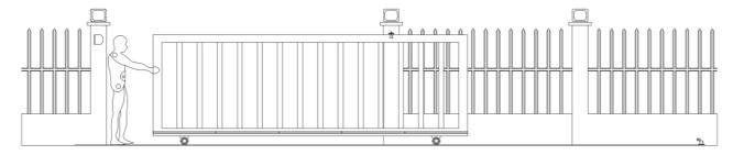
The gate should slide smoothly by hand before attempting to install the gate opener.
