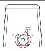
In manual mode, the gear can turn freely and the gate can be operated by hand.
