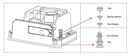
The bolts and flat washer between mounting plate and motor base are used for adjusting the height of the motor.
